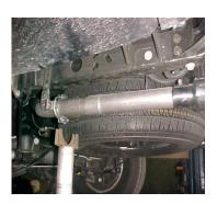
INSTALL EXIT PIPES # E. USE CLAMPS # G TO SECURE TO THE TAILPIPES. DO NOT TIGHTEN. USE ZIP TIES TO SECURE BRAKE AND FUEL LINES AWAY FROM EXHAUST.
