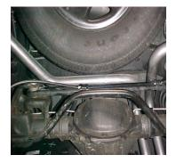
INSTALL THE PASSENGER SIDE OVERAXLE TAILPIPE #D TO THE MUFFLER 1-1/2"-2". USE CLAMP # G TO SECURE TAILPIPE TO MUFFLER. DO NOT TIGHTEN.
