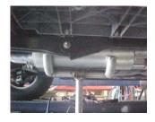
NEXT INSTALL MUFFLER #C. SLIDE IT ONTO
