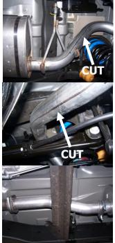
2. To remove the stock exhaust, unbolt it from the two bolt flange in front of the muffler. Do not disguard you will re-use bolts. Disengage the welded hangers using WD-40 from the OEM rubber grommets. Do not damage or remove the rubber grommets as you will reuse them to mount your new system. Now, cut off tailpipe before and after rear axle for removal.
