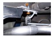
8. Now install driver side tailpipe hanger. Use same 1½" hole on the frame, but on the driver side. Install rubber grommet on hanger. Then install hanger from pipe into rubber grommet.
