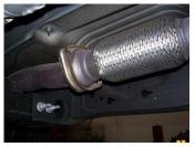
2. Remove the stock exhaust by unbolting it at the 2-bolt flange located in front of the muffler. Disengage the welded hangers from the OEM rubber grommets. Use WD-40 to aid in this process. Do not damage stock nuts and bolts or remove the rubber grommets as you will re-use them to mount your new system. Now, cut off tailpipe and remove system.
