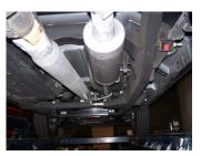
4. Install muffler #B onto headpipe  $1\frac{1}{2}$ "-2" with the louvers facing towards the converter. Use a jack stand to support the muffler. Use clamp #G to secure the muffler to the headpipe. Do not tighten. Muffler inlet is looking into the louvers.
