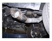
6. Slide passenger side tailpipe #C into muffler 1.5-2". Use clamp #H to secure. Do not tighten. Insert welded hangers into rubber grommets.
