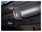
2. Remove the stock exhaust by unbolting it at the flange located in front of the muffler. Disengage the welded hangers from the OEM rubber grommets. Use WD-40 to aid in this process. Do not damage stock nuts and bolts or remove the rubber grommets as you will re-use them to mount your new system. Now, cut off tailpipe and remove system.
