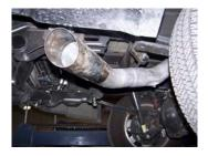
6. Slide passenger side tailpipe #C into muffler 1.5-2". Use clamp #H to secure. Do not tighten. Insert welded hangers into rubber grommets.
