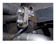
5. Next, remove your spare tire. Then install passenger side tailpipe hanger #I. You will see a 1½" hole in the frame. Attach hanger to this hole and re-install factory grommet on hanger.
