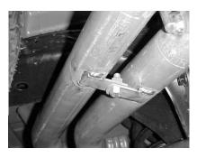
USING BOLT KIT #J AND ATTACH BOTH TAILPIPES. THE PASSENGER SIDE MOUNTING BRACKET WILL BE POSITIONED UNDERNEATH THE DRIVER SIDE.
