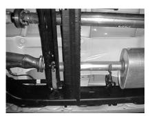
LAY OUT THE GIBSON EXHAUST AND COMPARE PART NUMBERS WITH THE MANUAL. FOR AN EASIER REMOVAL OF THE FACTORY EXHAUST CUT THE TAILPIPE BEHIND THE MUFFLER. THEN UN-BOLT THE FLANGE IN FRONT OF THE MUFFLER AND REMOVE. LEAVE ALL FACTORY RUBBER GROMMETS IN PLACE. YOU WILL RE-USE THE FACTORY BOLTS.
