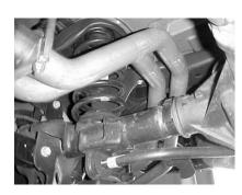
SLIP TAILPIPE #C INTO THE DRIVER SIDE OUTLET NO MORE THEN 2" AND NO LESS THEN 1". USE HANGER # E TO TIGHTEN THE CONNECTION AT THE MUFFLER OUTLET. DO NOT TIGHTEN
