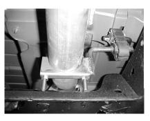
INSTALL HANGER # F ONTO HEADPIPE # A, AND INSERT WELDED HANGER INTO RUBBER GROMMET. DO NOT TIGHTEN.
