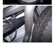
4. Install driver tailpipe #D onto muffler 11/2"-2". Route between shock and spare tire. Secure using clamp #I. DO NOT TIGHTEN. Insert welded hanger into rubber grommet.
