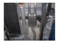
4. Install muffler #B with inlet towards Y-pipe. Use jack stands to support the muffler. Use clamp #F to secure the muffler to headpipe. Do not tighten.
