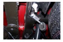
5. Install metal hanger #H into hole located approximately 16" from the rear of the frame. Use hardware kit #I, washer #M, and rubber grommet #J.
