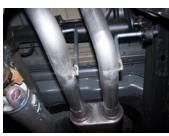
7. Using clamps #G secure both tailpipes to the outlets of the muffler. Rotate tailpipes to best fit your truck.
