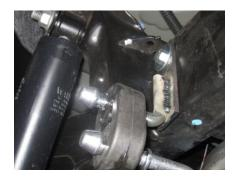
5.Next install drivers side rear hanger and gommet with bolt kit provided see picture the hanger goes on the outside of the frame and bolts through the whole frame
