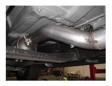
2.Install headpipe #A onto your factory pipe using your stock clamp insert welded hanger into the rubber grommet leave clamp loose.
