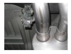
4.Next install Drivers side overaxle tailpipe #C into muffler 1.5" to 2" insert welded hanger into rubber grommet use clamp # F to secure pipe to muffler do not tighten
