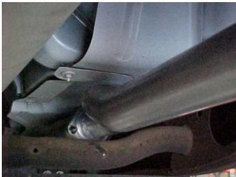
Install head pipe # A onto you're existing stock flange re-using the factory hardware. Use a jack stand to support the converter. Do not tighten. Insert welded hanger into rubber grommet.
