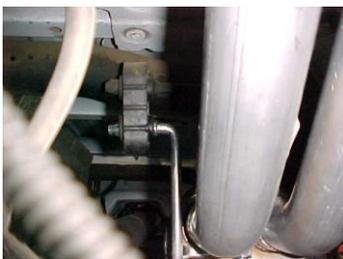
Install muffler # B onto head pipe 1-1/2" to 2" with the louvers facing towards the converter. Use a jack stand to support the muffler. Use clamp # G to secure the muffler to the head pipe. Do not tighten. Muffler inlet is looking into the louvers.
