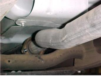
Lay out the exhaust on the floor so it looks like the drawing and compare parts with manual. To remove the stock exhaust un-bolt it from the flange located in front of the muffler. **You will re-use your stock hardware.** Leave all rubber grommets in place. Use WD-40 to aid in removal of exhaust and the hangers. Cut your stock tailpipe off just behind the muffler.
