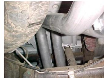
Install passenger side over axle tailpipe # C into muffler and attach using clamp # H. Use bolt kit # I to attach the tailpipes together. Do not tighten. YOU MAY NEED TO LOOSEN YOUR SPARE TIRE & PUSH TOWARDS DRIVER SIDE & RE-TIGHTEN
