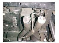
Install the passenger side over axle tailpipe # D into the muffler 1-1/2" to 2". Insert welded hanger into rubber grommet. Use clamp # J to secure pipe to muffler, do not tighten.
