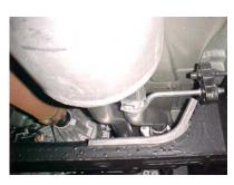
Install stainless steel tip. Clamp down.
