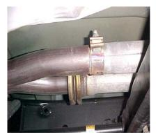
Lay out the exhaust on the floor so it looks like the drawing and compare parts with manual. To remove the stock exhaust remove it from the stock flange & slip joint located in front of the muffler, then cut off your tailpipe just behind the muffler.
