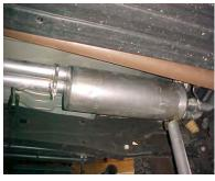
Install muffler #C onto head pipes #A-B 1-1/2" to 2" with the louvers facing towards the converter. Use a jack stand to support the muffler. Use clamps #G to secure the muffler to the head pipes. Do not tighten. Outlets of muffler should be on the bottom.
