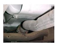
Lay out the exhaust on the floor so it looks like the drawing and compare parts with manual. To remove the stock exhaust remove it from the 2-bolt flange located in front of the new muffler. **Do not discard factory**hardware, you will reuse it. Leave all rubber grommets in place. Use WD-40 to aid in removal of exhaust and the hangers. Cut off tailpipe.
