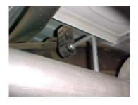
Install head pipe # A on to your existing stock front pipe and bolt using your factory bolts. Use a jack stand to support the converter. Insert welded hanger into rubber grommet.
