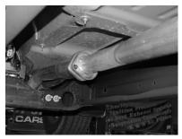
BOLT HEADPIPE #A TO STOCK FLANGE RE-USING FACTORY NUTS. DO NOT TIGHTEN AND CONNCET WITH CLAMP #F. SLIDE WELDED HANGER INTO RUBBER GROMMET.INSTALL HEAD PIPE EXTENSION #J.
