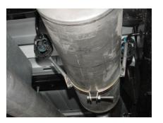
INSTALL MUFFLER #B ONTO HEADPIPE 1-1/2" TO 2". USE CLAMP #I TO SECURE THE MUFFLER TO THE HEADPIPE. DO NOT TIGHTEN. SLIDE BAND CLAMP #J ONTO THE MUFFLER AND INSERT THE WELDED HANGER INTO THE RUBBER GROMMET.
