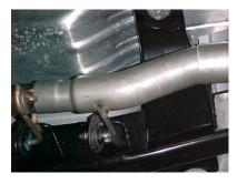
UNCLAMP THE STOCK EXHAUST JUST IN FRONT OF THE MUFFLER. YOU MAY NEED TO HEAT IT UP FOR EASIER REMOVAL. LEAVE ALL RUBBER GROMMETS IN PLACE. USE WD-40 TO AID IN REMOVAL OF EXHAUST AND HANGERS.
