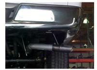
INSTALL PASSENGER SIDE TAILPIPE #C INTO MUFFLER 1-1/2" TO 2". USE CLAMP #G TO SECURE TAILPIPE TO MUFFLER. INSERT WELDED HANGER INTO RUBBER GROMMET. DO NOT TIGHTEN.
