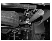
WASHER WILL GO INTO THE 1<sup>27</sup> HOLE FROM THE TOP OF THE HANGER. INSTALL DRIVER SIDE TAILPIPE #D INTO MUFFLER AT LEAST 1 ½" TO 2". THIS PIPE WILL ROUTE OVER THE AXLE AND BETWEEN THE SHOCK AND TIRE. ATTACH CLAMP # HTO SECURE PIPE TO MUFFLER. DO NOT TIGHTEN. LOOKING FROM THE REAR OF THE VEHICLE - THIS TAILPIPE IS
