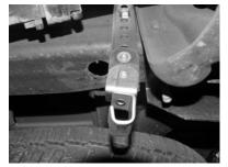
INSTALL METAL HANGERS # J INTO SLOTTED HOLES LOCATED APPROX. 16" FROM THE REAR OF THE FRAME. METAL HANGERS ARE MOUNTED ON THE OUTSIDE OF FRAME. USE THE HARDWARE THE PROVIDED. THE BOLT AND WASHER WILL GO INTO THE 1<sup>ST</sup> HOLE FROM THE TOP OF THE HANGER.
