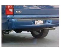
**INSTALL EXIT PIPES # F ONTO** TAILPIPES. CUT TO YOUR PREFERED LENGTH USE CLAMPS # I TO SECURE EXIT PIPES TO TAILPIPES. THESE CLAMPS ALSO ATTACH TO METAL HANGERS # J. THESE METAL HANGERS NEED TO BE ROTATED IN ORDER TO ADJUST FOR CLAMPING. ROTATE EXIT PIPES TO POINT OUT TO THE SIDE, NOW YOU CAN TIGHTEN ALL CLAMPS, NUTS, AND BOLTS. STARTING FROM THE FRONT WORKING BACK. INSTALL STAINLESS TIPS. USE ZIP TIES FOR BRAKE AND FUEL LINES.
