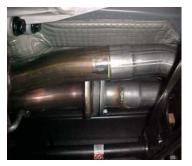
INSTALL PASSENGERSIDE HEADPIPE #A ONTO FACTORY FLANGE USING THE HARDWARE # K. DO NOT TIGHTEN. INSERT HANGER INTO RUBBER GROMMET. NEXT, INSTALL DRIVERSIDE HEADPIPE #B ONTO THE FACTORY PIPE. USE CLAMP # I TO SECURE. DO NOT
