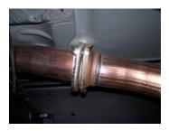
**2.** To remove the stock exhaust, unbolt the head pipe at the 2 bolt flange. Disengage the welded hangers using WD-40 from the OEM rubber grommets. Do not damage or remove the rubber grommets as you will reuse them to mount your new system.
