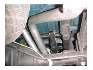
**8.** Install passenger side over axle tail pipe #C into muffler 1½-2". Secure with clamp #G. Do not tighten.
