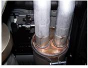
**4.** Slide muffler #B onto head pipe #A 1½"-2" with the louvers facing towards the converter. Use a jack stand to support the muffler. Use clamp #I to secure the muffler to the head pipe. Do not tighten. Install band clamp #J onto muffler. Insert hanger on band clamp into rubber grommets. Use bolt kit provided. Do not tighten.
