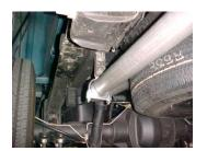
**9.** Install tail pipe hangers #H onto end of tail pipes using clamp #G. There will be about a 2" hole above the end of both tail pipes on the frame to bolt the hangers. Do not tighten.
