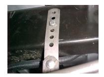
MEASURE 19 ½" FROM THE REAR OF THE FRAME AND USE THIS HOLE AND BOLT ON HANGER #H. USE THE 2<sup>ND</sup> HOLE FROM THE TOP.
