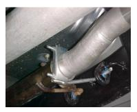
INSTALL HEADPIPE #A, YOU WILL NEED TO LINE UP THE TWO NOTCHES. USE FRONT HANGER #L TO SECURE PIPES TOGETHER AND INSERT HANGER INTO RUBBER GROMMET. DO NOT TIGHTEN.
