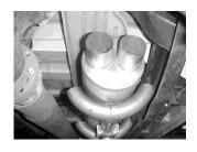
INSTALL MUFFLER ONTO STOCK HEADPIPE AND ATTACH WITH CLAMP #E. ALIGN NOTCH ON MUFFLER TO STOCK ALIGNMENT PIN ON FACTORY HEADPIPE. MUFFLER INLET IS TOWARDS THE CONVERTER. USE A JACK STAND TO SUPPORT THE MUFFLER.
