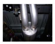
4. Install muffler #B onto headpipe 1.5-2" with the louvers facing towards the converter. Use a jack stand to support the muffler. Use clamp #G to secure the muffler to the headpipe. Do not tighten. Muffler inlet is looking into louvers.
