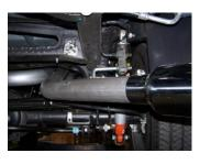
6. Install passenger side tailpipe #C into muffler 1.5-2". Use clamp #H to secure pipes together. Do not tighten. Insert welded hanger into rubber grommet.
