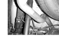
INSTALL THE DRIVER SIDE TAILPIPE #D INTO THE MUFFLER AND LEAST 1-1/2" TO 2". THIS PIPE WILL ROUTE OVER THE AXLE, BETWEEN THE SHOCK AND TIRE. USE CLAMP #J TO SECURE THE PIPE TO THE MUFFLER. **DO NOT TIGHTEN.** THEN, INSERT THE HANGERS INTO THE RUBBER GROMMETS.
