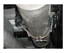
INSTALL MUFFLER #B ONTO HEADPIPE #A 1-1/2" TO 2". USE CLAMP #I TO SECURE THE MUFFLER TO THE HEADPIPE. DO NOT TIGHTEN. SLIDE BAND CLAMP #J ONTO THE MUFFLER AND INSERT THE WELDED HANGER INTO THE RUBBER GROMMET AND ATTACH TO MUFFLER WITH BOLT KIT #K.
