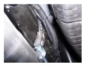
**6.** Measure 19<sup>1</sup>/<sub>2</sub>" from the rear of the frame. Use the third hole from the top to attach 10" hanger #H with bolt kit #I. DO NOT TIGHTEN.
