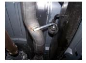
**2.** Install head pipe #A onto your existing stock front pipe and attach with clamp #J. Use a jack stand to support the converter. Insert welded hanger into rubber grommet.
