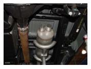
4. SLIDE MUFFLER #C ONTO HEADPIPES 1-1/2" TO 2" WITH THE INLET FACING THE MOTOR, USE A JACK STAND TO SUPPORT MUFFLER. USE CLAMPS # J TO SECURE MUFFLER TO HEADPIPES. DO NOT TIGHTEN. OUTLETS OF THE MUFFLER SHOULD BE ON THE TOP.
