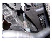
6. MEASURE 18" FROM THE REAR OF THE FRAME TOWARDS THE FRONT OF THE VEHICLE. USE THIS SLOT FOR THE 10" HANGER #K, INSTALL USING THE 1ST HOLE USE HARDWARE KIT #L.
