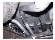
7. INSTALL PASSENGER SIDE OVER AXLE TAILPIPE #E INTO MUFFLER 11/2" TO 2" INSERT WELDED HANGER INTO RUBBER GROMMET. USE CLAMP # J TO SECURE PIPE TO MUFFLER. DO NOT TIGHTEN.
