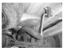
Install the Passenger side over-axle tailpipe # C to the muffler, 1-1/2" to 2". Use clamp # I to secure the tailpipe to the muffler.
