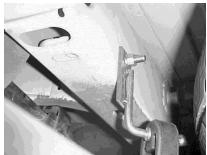
Install tailpipe hanger #J on the frame, then measure 9" from the rear; you will see a 1" round hole use this to mount your hanger. Use the bolt kit and rubber grommet provided in your kit.
