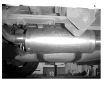
Install muffler #B onto head-pipe #A 1-1/2" to 2" with the louvers in the muffler facing towards the converter. Use a jack stand to support the muffler. Use Clamp #G to secure the muffler to the head-pipe. **Do Not Tighten at this Time!**
