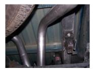
6. Install the passenger side over axle tailpipe #C into the muffler 1.5-2". Use clamp #H to secure. Do not tighten. Insert welded hanger into rubber grommet.
