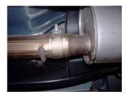
2. To remove stock exhaust, unclamp just in front of the muffler. Do not remove stock headpipe. Disengage the welded hangers from the rubber grommets. Use WD-40 to aid in this process. Do not damage or remove the rubber grommets as you will re-use them to mount your new system.
