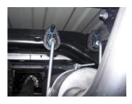
5. Slide band clamp #J onto muffler #B and attach with bolt kit #L. Do not tighten. Insert hangers into rubber grommets.
