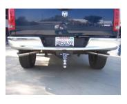
9. Install stainless steel tips. Clamp down. When you have everything in place, firmly tighten all bolts and clamps down securely. Use stainless steel cleaner and a Scotch Brite pad weekly to prevent tip from discoloration. Inspect all fasteners after 25-50 miles of operation and re-tighten as necessary.
