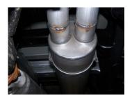
4. Install muffler #B onto headpipe #A 1.5-2" with the louvers facing towards the converter. Use a jack stand to support the muffler. Use clamp #I to secure the muffler to the headpipe. Do not tighten. Muffler inlet is looking into the louvers.
