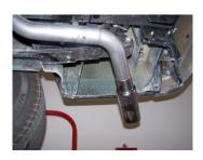
8. Install exit pipes #E onto tailpipes and secure with clamps #H. Do not tighten.
