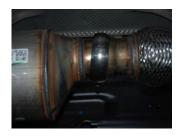
2. To remove stock exhaust, unbolt it from the flange behind the Y-pipe. Make sure to leave all rubber grommets in the factory location. You will re-use stock clamp. For easier removal of exhaust, cut behind the muffler. Use WD-40 to remove hangers from grommets.
