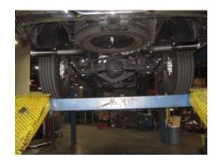
7. Install exit pipes #E onto tailpipes use clamp # F to secure together. After everything is installed begin to tighten all connections starting from the furthest forward connection. Items will move as you tighten. Be sure to check all clearance.
