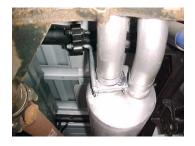
Install muffler #C onto head pipe #B 1-1/2" to 2" with the louvers facing towards the converter. Use a jack stand to support the muffler. Use clamp #G to secure the muffler to the head pipe. Do not tighten. Install rear muffler hanger #I onto driverside muffler outlet. Insert hanger into rubber grommet. Do not tighten.
