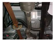
Install head pipe #A onto you're existing stock flange using your factory hardware. Do not tighten. Next slide headpipe #B onto headpipe #A. Insert welded hanger into rubber grommet. Use clamp #G to secure pipes together. Do not tighten.
