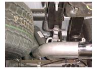
Install the passenger side over axle tailpipe #D into the muffler  $1 \frac{1}{2}$ " to 2". Use clamp #H to secure tailpipe to muffler. Do not tighten. Insert welded hanger into rubber grommet
