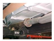
Lay out the exhaust on the floor so it looks like the drawing and compare parts with manual. To remove the stock exhaust un-bolt it from the 2-bolt flange located behind your factory Y-pipe. You will re-use your factory hardware. Leave all rubber grommets in place. Use WD-40 to aid in removal of exhaust and the hangers. Now cut off your stock tailpipe just behind the muffler.
