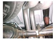
Install driver side over axle tailpipe #E into muffler and attach using clamp #I. Use bolt kit #J to attach the tailpipes together. Do not tighten. Driverside pipes tab will be on the bottom when putting bolting pipes together.
