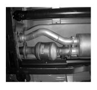
INSTALL HEADPIPE #A ON THE FACTORY DRIVERSIDE AND ATTACH HEADPIPE USING CLAMP #F. DO NOT TIGHTEN. INSTALL THE MUFFLER WITH THE OUTLET'S POSITIONED AT 12 O'CLOCK. INLET HAS LOUVERS FACING FORWARD TO CATCH THE EXHAUST. USE A JACKSTAND TO SUPPORT THE MUFFLER.
