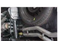
Install the driver side over axle tailpipe #D into the muffler 1-1/2" to 2". Use clamp #H to secure tailpipe to muffler. Use bolt kit #I to secure tailpipes #D & E together. Driver side tailpipe will have tab on bottom. Do not tighten.
