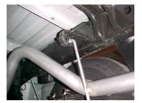
INSTALL MUFFLER #B ONTO HEADPIPE 1-1/2" TO 2". USE CLAMP #H TO SECURE THE MUFFLER TO THE HEADPIPE. INSERT WELED HANGER INTO RUBBER GROMMET. DO NOT TIGHTEN. SLIDE BAND CLAMP #I ONTO THE MUFFLER AND INSERT THE WELDED HANGER INTO THE RUBBER GROMMET. ATTACH WITH BOLT KIT # J.
