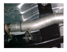
**INSTALL HEADPIPE #A,** YOU WILL NEED TO LINE UP THE TWO NOTCHES. USE CLAMP #K TO SECURE HEADPIPE TO THE STOCK PIPE. DO NOT TIGHTEN. **INSERT HANGER INTO**
