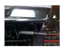
INSTALL EXIT PIPES #E, USE CLAMPS #G TO SECURE TO THE TAILPIPES.
