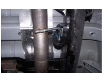
INSTALL HEADPIPE #A, YOU WILL NEED TO LINE UP THE TWO NOTCHES. INSERT WELDED HANGER INTO RUBBER GROMMET, USE CLAMP #G TO SECURE HEADPIPE TO THE STOCK PIPE. DO NOT TIGHTEN.
