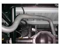
**INSTALL DRIVER SIDE** TAILPIPE #D INTO MUFFLER 1-1/2" TO 2" AND USE CLAMP #G TO SECURE TO THE MUFFLER. DO NOT TIGHTEN. USE CLAMP #G TO HOLD PIPE UP TO THE HANGER #H. DO NOT TIGHTEN.
