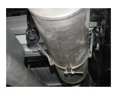
INSTALL MUFFLER #B ONTO HEADPIPE #A 1-1/2" TO 2". USE CLAMP **#I TO SECURE THE** MUFFLER TO THE HEADPIPE, DO NOT TIGHTEN. SLIDE BAND CLAMP #J ONTO THE MUFFLER AND INSERT THE WELDED HANGER INTO THE RUBBER GROMMET AND ATTACH TO MUFFLER WITH BOLT KIT #K.
