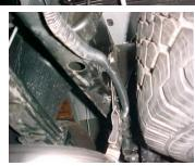
MEASURE 19 1/2" FROM THE REAR OF THE FRAME AND USE THIS HOLE AND BOLT ON HANGER #H ON THE INSIDE OF FRAME #H. USE THE 2ND HOLE FROM THE TOP.
