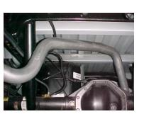
**INSTALL DRIVER SIDE** TAILPIPE #D INTO MUFFLER 1-1/2" TO 2" AND USE CLAMP #G TO SECURE TO THE MUFFLER. DO NOT TIGHTEN. USE CLAMP #G TO HOLD PIPE UP TO THE HANGER #H. DO NOT TIGHTEN.
