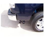
9. INSTALL YOUR BLACK CERAMIC COATED TIPS. PROCEED TO THE NEXT SHEET ON HOW TO INSTALL YOUR DEEGAN 38 BADGES. AFTER YOU HAVE CHECKED FOR CLEARANCES GO BACK AND TIGHTEN ALL NUTS, BOLTS AND CLAMPS.
