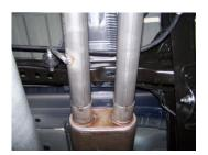
4. Install muffler onto headpipes 1.5"-2" with the louvers facing towards the converter. Use a jack stand to support the muffler. Use clamps #J to secure the muffler to the headpipes. Do not tighten. Muffler inlet is looking into the louvers.
