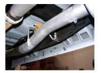
INSTALL HEADPIPE # A ONTO FACTORY PIPE. LINE UP THE NOTCH. USE CLAMP # G TO SECURE HEADPIPE TO FACTORY PIPE. DO NOT TIGHTEN. INSERT WELDED HANGER INTO RUBBER GROMMET.
