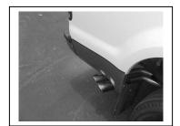
INSTALL YOUR BLACK CERAMIC COATED TIPS. PROCEED TO THE NEXT SHEET ON HOW TO INSTALL YOUR DEEGAN 38 BADGES. AFTER YOU HAVE CHECKED FOR CLEARANCES GO BACK AND TIGHTEN ALL NUTS,
