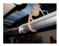
TO REMOVE YOUR STOCK EXHAUST, UNBOLT AND REMOVE IT FROM THE SECOND CLAMP LOCATED JUST IN FRONT OF THE MUFFLER. FOR EASIER REMOVAL OF THE FACTORY EXHAUST, CUT OFF THE STOCK TAILPIPE JUST BEHIND THE MUFFLER AND REMOVE. LEAVE ALL RUBBER GROMMETS ON THE HANGERS. USE WD-40 TO AID IN REMOVAL OF EXHAUST AND HANGERS.
