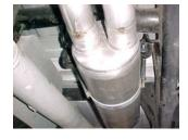
Lay out the exhaust on the floor so it looks like the drawing and compare parts with manual. To remove the stock exhaust un-clamp it just in front of the muffler. Leave all rubber grommets in place. Use WD-40 to aid in removal of exhaust and the hangers.
