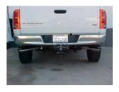
Measure 18" from the rear of the frame and install the rear tailpipe hanger #K on outside frame rail, using rubber grommet #J and bolt kit #L to secure. Do not tighten.
