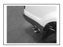
INSTALL YOUR STAINLESS TIPS. TIGHTEN ALL CLAMPS STARTING FROM THE FRONT, WORKING YOUR WAY TO THE BACK OF THE TRUCK. TO CLEAN TIPS USE A STAINLESS STEEL CLEANER & SCOTCH BTIE PAD.
