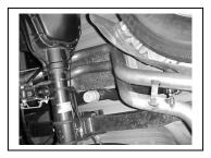
NEXT INSTALL DRIVERS OVER AXLE PIPE # D INTO MUFFLER 1½ TO 2". USE CLAMP # F TO SECURE PIPE TO MUFFLER. DO NOT TIGHTEN. USE BOLT KIT # I TO SECURE PIPES TOGETHER. DRIVERSIDE TAB WILL BE ON THE BOTTOM.
