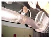
1. To remove the stock exhaust remove it from the clamp located in front of the stock muffler. Disengage the welded hangers using WD-40 from the OEM rubber grommets. Do not damage or remove the rubber grommets as you will re-use them to mount your new system. Now, cut off tailbibe and remove exhaust.
