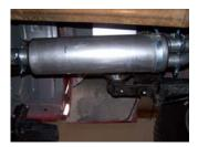
**3.** Install muffler #B onto head pipe #A 1½"-2" with the louvers facing towards the converter. Use a jack stand to support the muffler. Use clamp #G to secure the muffler to the headpipe. Do not tighten. Muffler inlet is looking into the louvers.
