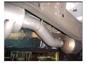
2. Install headpipe #A onto your catalytic converter and attach with clamp #K. Use a jack stand to support the converter. DO NOT TIGHTEN. Insert welded hanger into rubber grommet.
