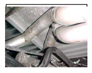
**4.** Install driver side over axle pipe #C into the muffler  $1\frac{1}{2}$ -2" and secure with clamp #H. DO NOT TIGHTEN.
