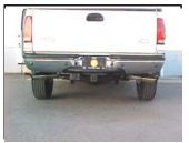
**8.** Install stainless steel tips #F. Clamp down. When you have everything in place, firmly tighten all bolts and clamps down securely. Use stainless steel cleaner and a Scotch Brite pad weekly to prevent tip from discoloration.
