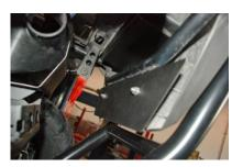
3. Next install Item # F and Item # B. You will use the supplied bolts to bolt both plates together. The polished rear plate will be on the outside of the vehicle and Item # F is the heat shield on the inside of the rear valance designed to protect the rear plastics.
