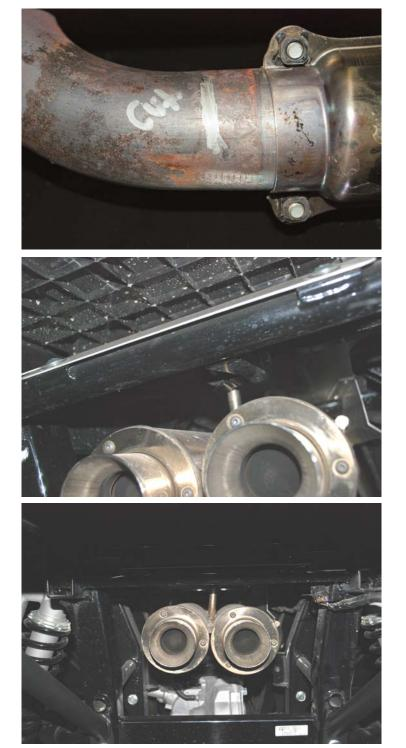
To begin the install of the Gibson Performance exhaust you will need to remove the factory rear portion of the skid plate. This will allow access to the factory head pipe where you will need to cut your header. You will measure 2" rear of the heat shield towards the back of the vehicle. This is the last heat shield before the exhaust makes the up turn towards the bottom of the vehicle.
