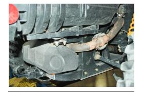
Remove your factory exhaust system for the donut flange connection located on the passenger side in front of the muffler. Do not damage springs or gasket they will be re used in the install of the new Gibson system.
