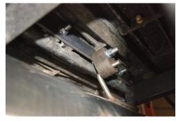
Install the hanger bracket using the supplied bolt kit. This bracket will also support the supplied rubber grommet.
