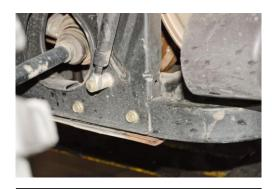
Begin the removal of the factory exhaust by removing the factory hitch; there are a total of four bolts two on each side. Removing the factory skid plate will make for an easier removal of the hitch but is not a necessary step.
