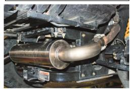
Use the factory gasket and springs for the install of the Gibson exhaust.
