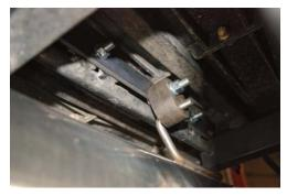
Install the hanger bracket using the supplied bolt kit. This bracket will also support the supplied rubber grommet.
