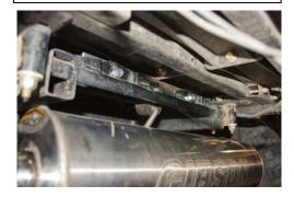
With the rubber grommet and the bracket securely tightened down install the muffler assembly.
