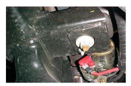
7. IT IS NOT NECESSARY TO REMOVE THE INNER FENDERWELLS, BUT IT MAKES THE INSTALL EASIER ON THE PASSENGER SIDE. TO REMOVE THE FENDERWELLS SIMPLY UNSCREW ALL THE SHEET METAL SCREWS AND FASTENERS ATTACHING IT TO THE FENDER AND FRAME AND THE FENDERWELL WILL DROP OUT.
